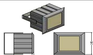
4watt, 2 led, 664lm (equiv. Alogeno 30w), Apert. Fascio 45°, 220vac
